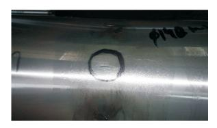
Any Magnetic particle build up having width more than 1.0mm and ratio of length to width more than three times will mean defect/crack.
