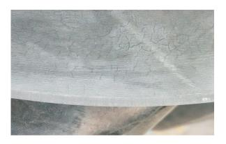
pressure. When applied on roll surface the softer areas will darken faster than the surroundings leaving a differential etch appearance. Cracks are also highlighted during an etching test. The reagent that enters the crack interface through capillary action. when the acid is cleaned the residual acid seeps out within the cracks and burns the area surrounding it. this test is also supplemented by UT testing on the located surface.
